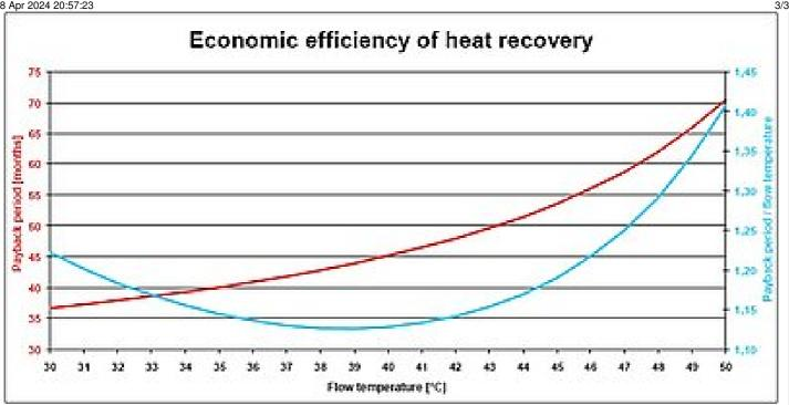
The blue curve describes the payback period / flow temperature ratio. The optimal operating point is achieved with a low payback period and high temperature within the heating circuit. The quotient of both values has therefore its lowest value at the optimal operating point. The diagram shows this value at approx. 39°C. The optimal temperature for a heating plant with heat pump lies between 35° and 45°. This fact is underlined by the figures provided by the diagram.
