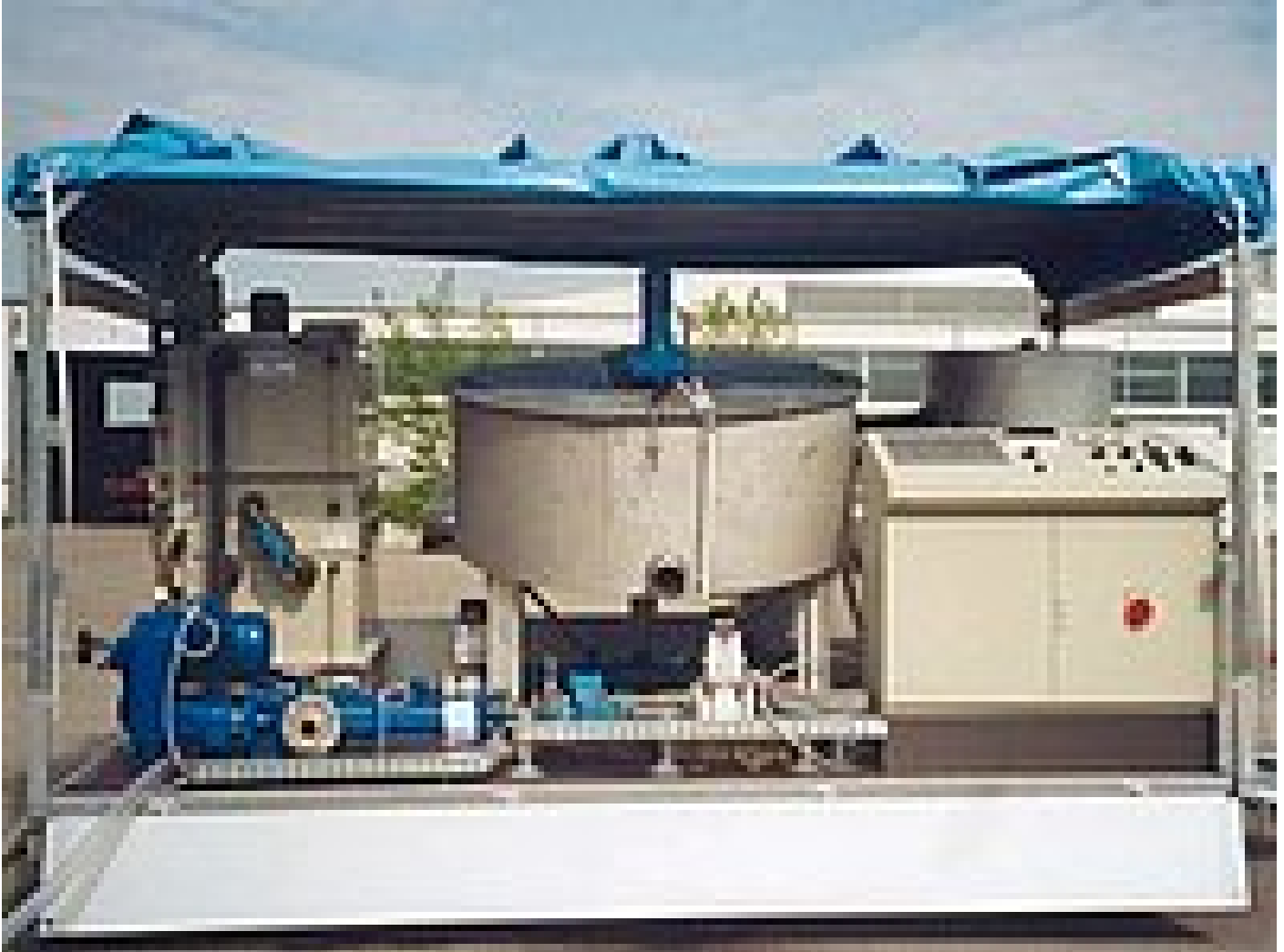
Trailer-mounted ROTAMAT® disc thickener RoS 2S
