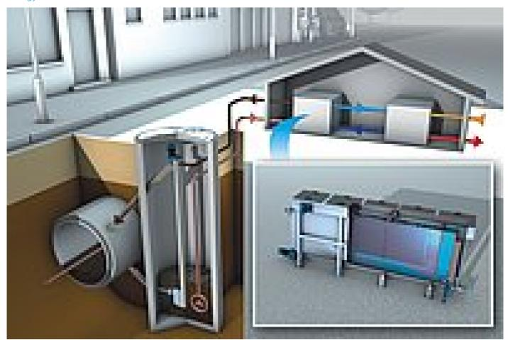
Wastewater contains thermal energy, and we can recover some of this energy with heat pumps.
