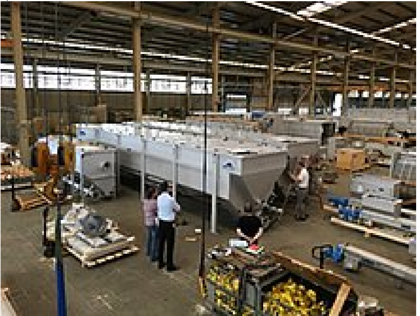
Figure 2 - DuPont DAF factory acceptance test in Germany at the production site
