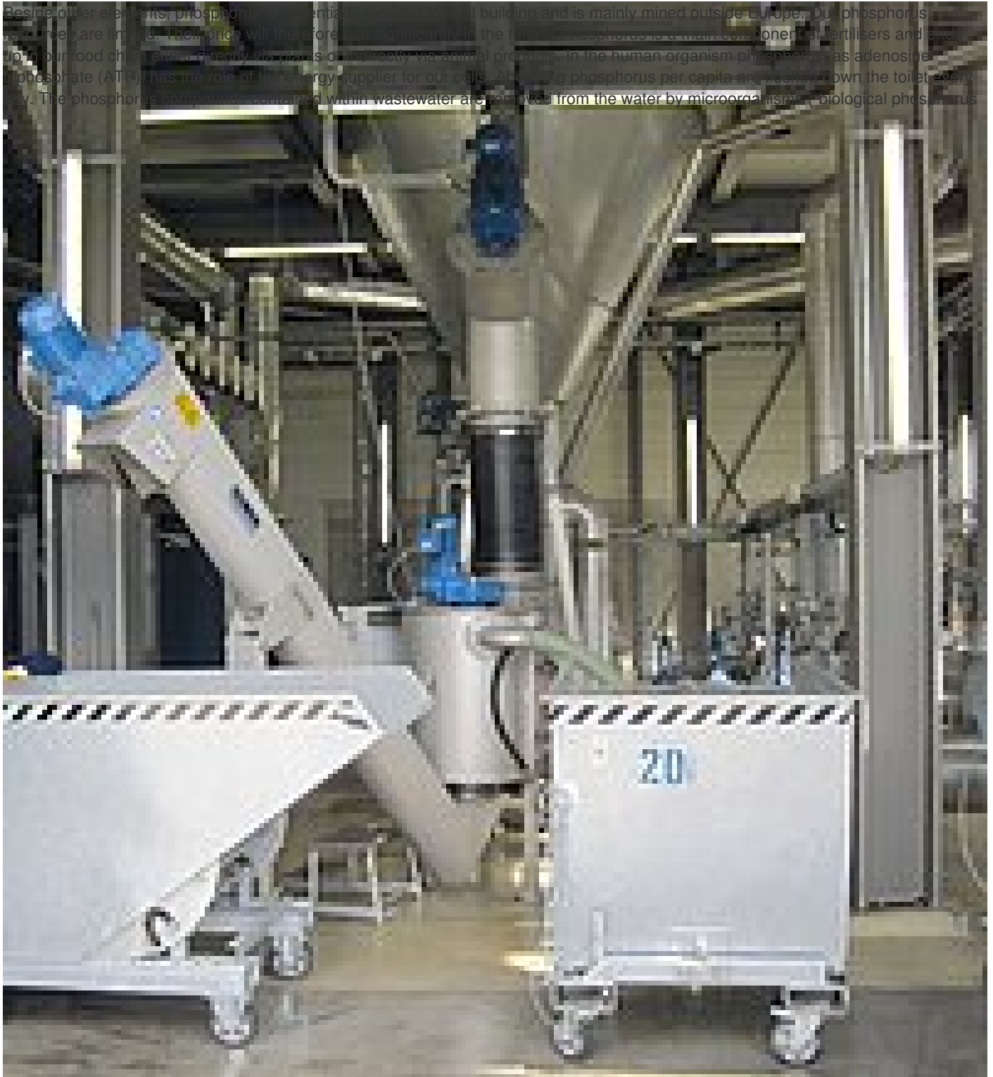
HUBER Grit Washer RoSF4/t for selective removal of MAP crystals from sewage sludge
