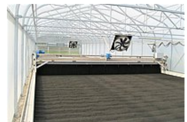
HUBER Sludge Turner SOLSTICE®
