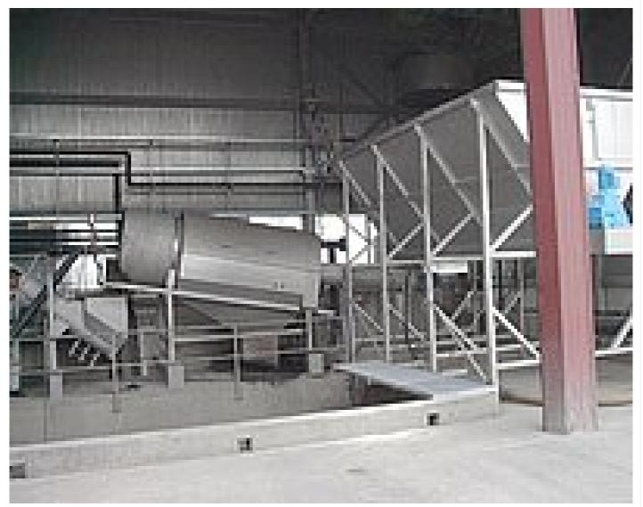
Treatment of grit from wastewater treatment plants, sewer systems and of refuse and oil grit by means of a Wash Drum / Grit Washer
