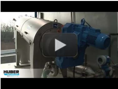
Video: HUBER Screw Press Q-PRESS@ - here at a municipal WWTTP
